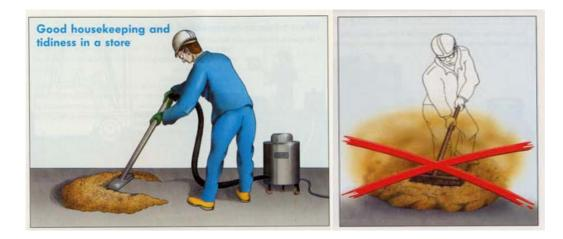
Figure 3.2: Removal of dust deposits<sup>4</sup>
