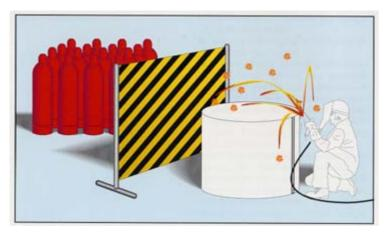
Figure 4.2: Example of screening for work giving rise to flying sparks<sup>4</sup>
