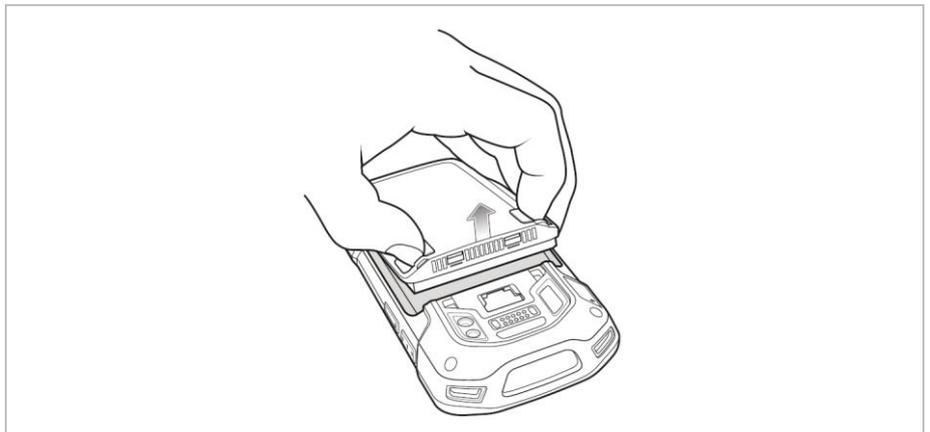
9. Insert the replacement battery, bottom first, into the battery compartment in the back of the device.
