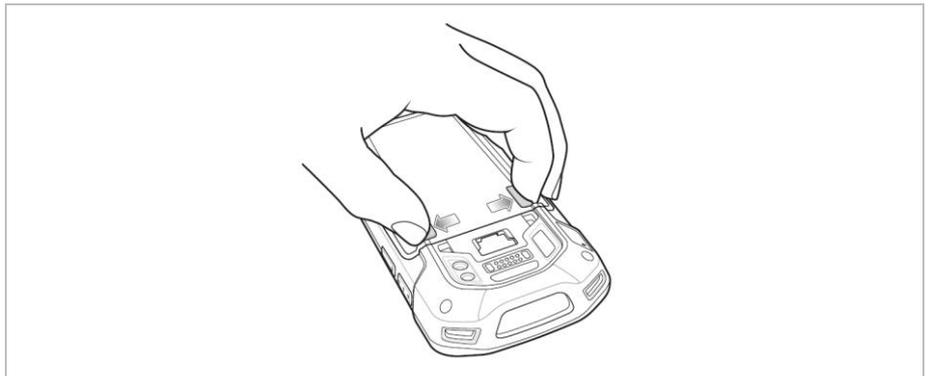
8. Lift the battery from the device.
